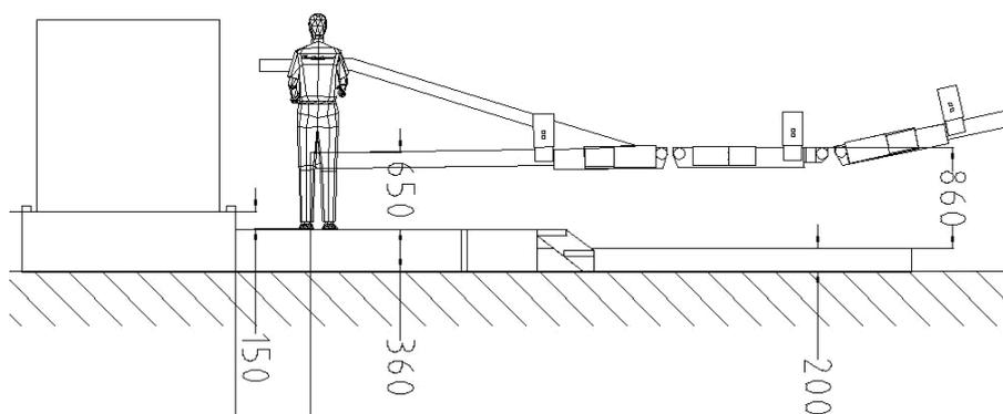
Figure 2. Sketch of extended belt loader (EBL).
