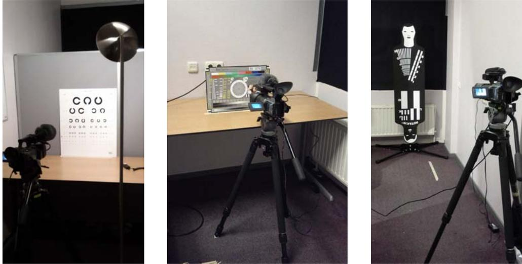
Figure 3. Three test conditions for Landolt C, Vidilabs and Rotakin test charts.
